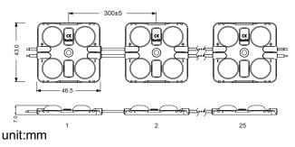
Note: the pitch based on 260mm Wire
