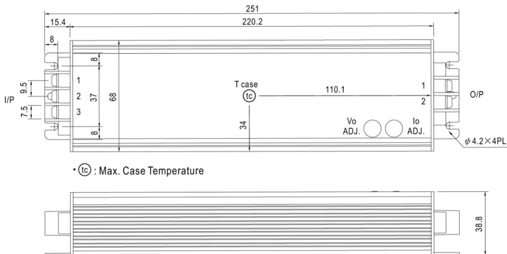
AC Input Terminal Pin No. Assignment
